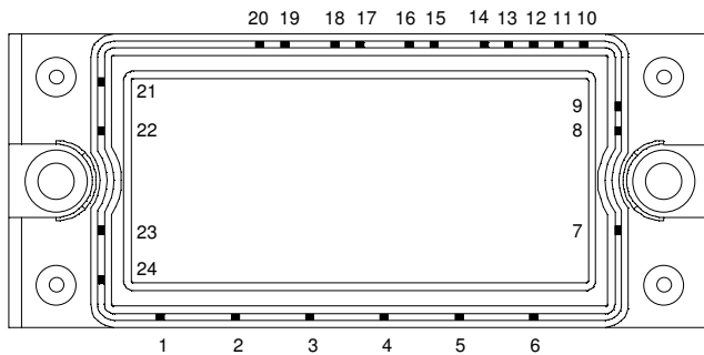
APTGS10X120RTP2: Without Brake (Pin 7 & 14 not connected)
